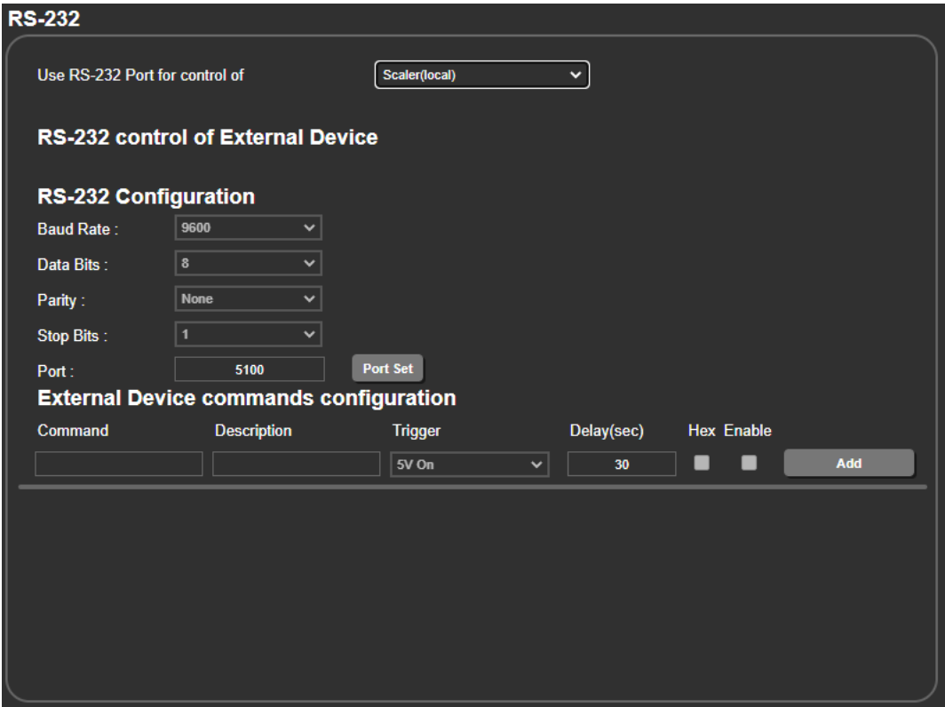
Figure 28: RS-232 Page – Controlling the VP-427X1
