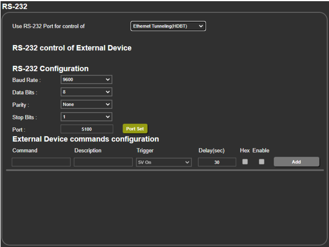
Figure 41: RS-232 Page – Controlling an External Device
