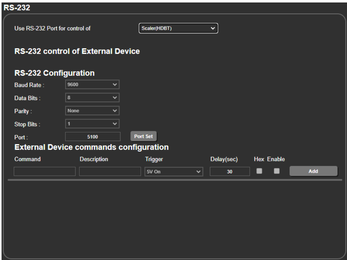
Figure 39: RS-232 Page – Controlling an External Device via HDBT Tunneling
